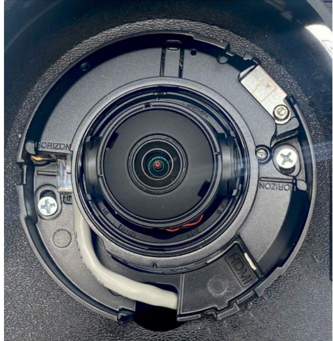
With the lens cover removed, you can adjust the camera head for the best view.
