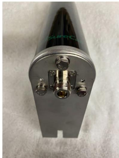
Antenna attached to T-post bracket, bottom view
