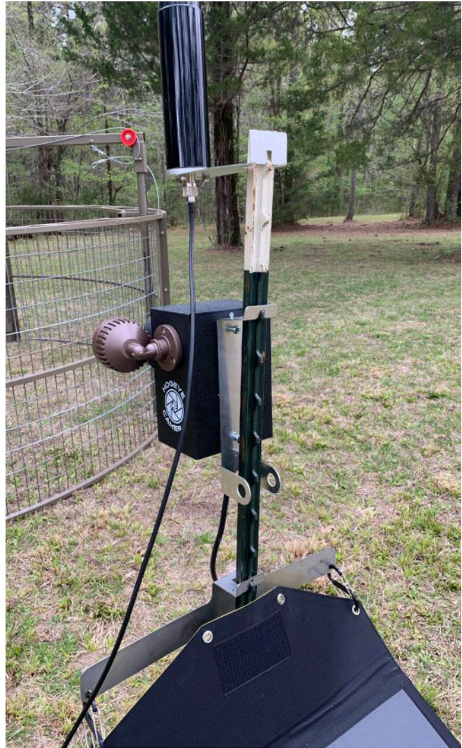
Solar panel, camera, and antenna on T-post
