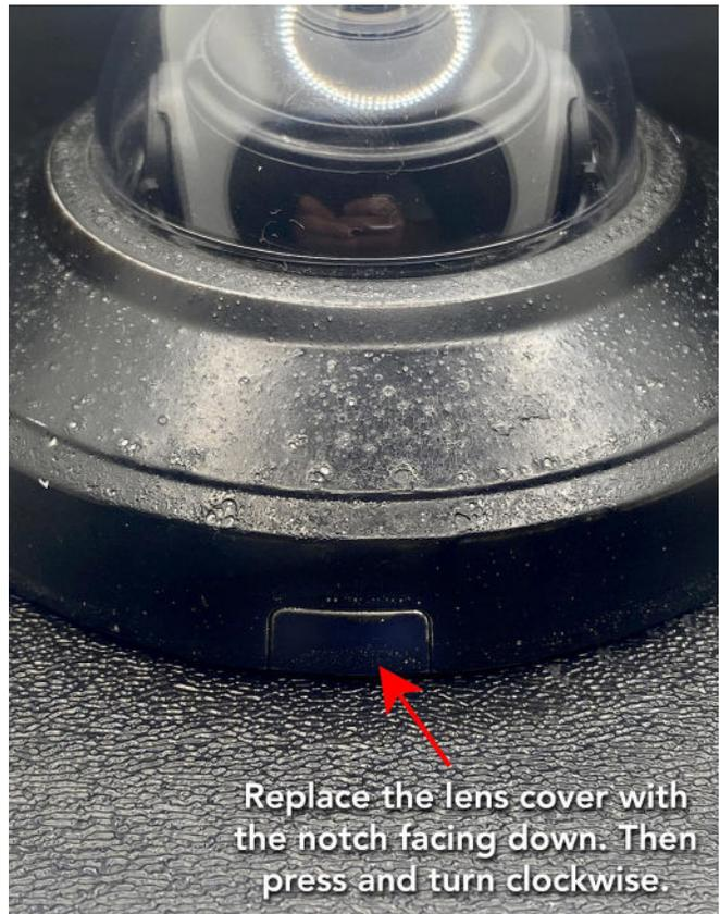
Make sure the notch on the lens cover faces the bottom of the camera when you replace it.
